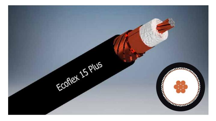
Ecoflex 15 Plus has remarkably improved electrical and mechanical characterisitics. The construction of the cable and the use of materials are optimized to achieve lowest attenuation values, higher max. frequency, high long-term stability and low weight, also allowing an easy installation.
