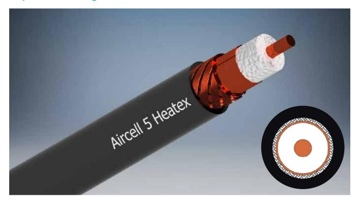
Aircell 5 Heatex is a flexible and thin coaxial cable with 5 mm outer diameter for the frequency range from DC to 10 GHz. Its low loss characteristics in relation to the diameter and the ability to use standard RG 58 connectors make this cable the number one choice not only for Wireless LAN applications but also for general RF communications.
